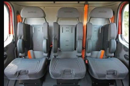
The roomiest cab in its class features high headroom allowing firefighters to wear their helmets in the truck. SCBA seats are also available for the crew.
